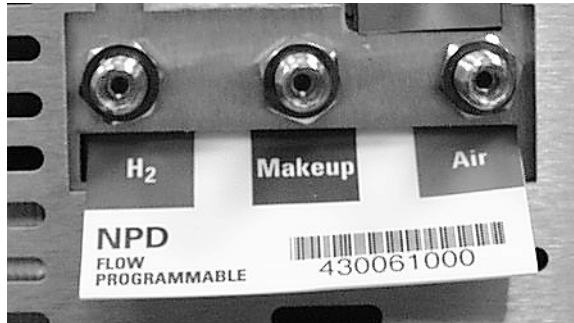
Figure 5. Gas line connections
